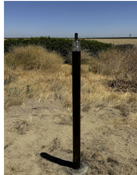
Figure 6 - Permanent Mounting Post for GNSS Receiver
